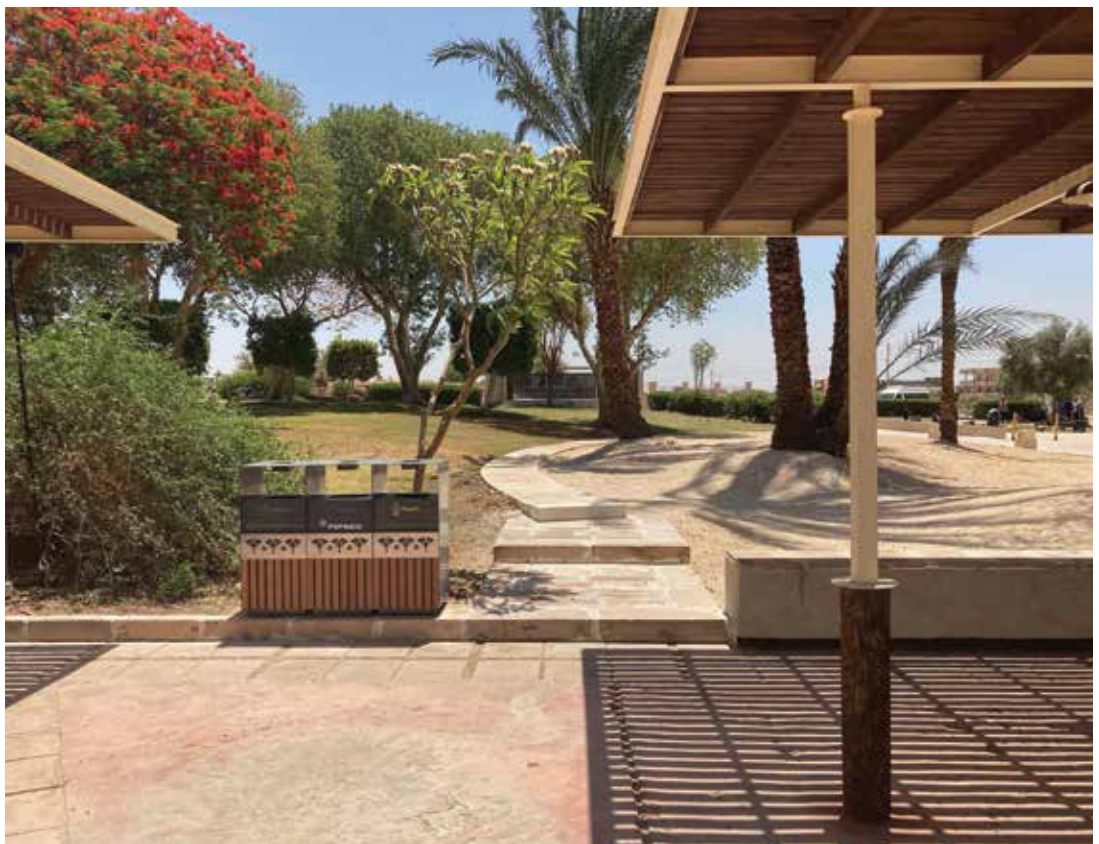
On the northwest side of the house damaged cement panels were replaced with sandstone paving, sandstone curbs, and masonry benches. Also pictured are new shading structures constructed from steel frames and timber cladding.
